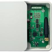
Heatit Z-Relay multipurpose relay module may be used for many different applications. The IP 55 rated casing makes it useful for any outdoor application. Can pull loads up to 25A.
